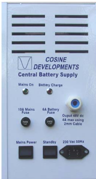
Figure 3: A Central Battery Base Station
